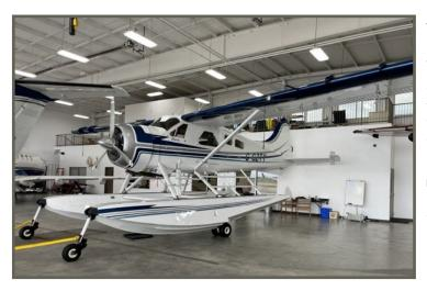
The airframe was stripped of paint during the rebuild and the majority of skins replaced. A Wipline 5600 lb. gross weight STC and Sealand extended baggage with Alaska Door was installed. The birdcage was removed and inspected. The birdcage was again inspected in July 2019. All fuel and oil hoses were replaced. The wiring was replaced with all new switches and circuit breakers. New Kenmore fuselage (windshield) struts were installed. New life-time wing struts installed.
